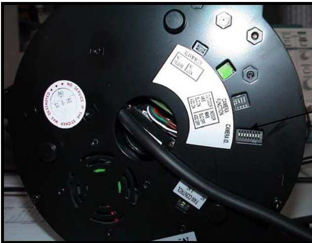
Figure: Base of the Lilin Domes with address switch S1
